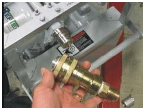
...Quick connect kit (KIT001) may be purchased separately & installed to flare connections on Lovac & hoses.
